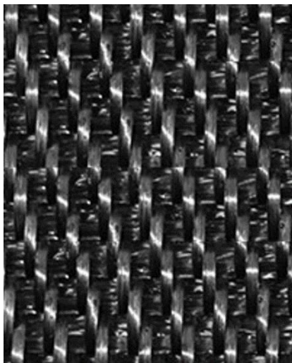
Fig 3. Woven mono-filament fabric
