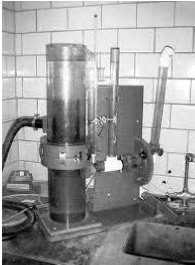
Fig 10. ASTM D4491 Geotextile permeability test
