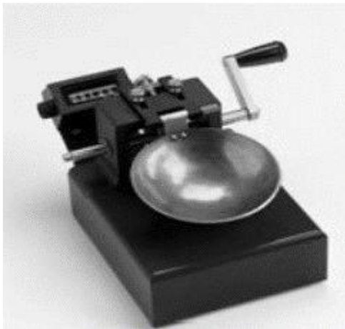
Fig 8. ASTM D4318 Atterberg limits
