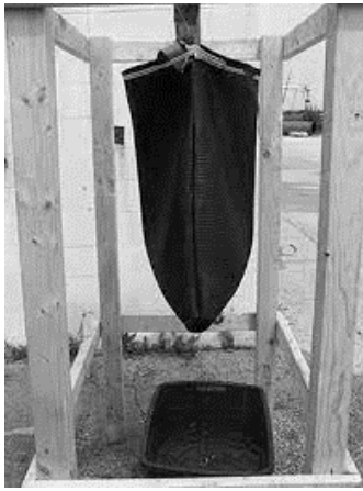
Fig 11. Hanging bag test ASTM D7701
